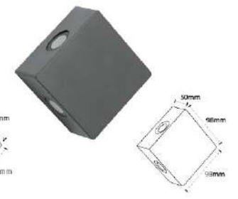
SL 2004 - Round Lens LED : 1x3W, 2x3W, 3x3W, 4x3W Color Temperature : 3000K, 6000K Material: Die-casting Aluminium with Toughened Glass Body Color: Graphite Gray
